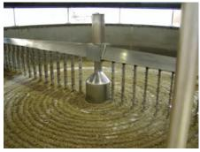
Mashing the Grist. The dry malt, once out of the kiln is ready to be put through a mill which grinds it into a rough powder.
